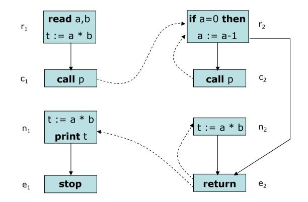
The following call strings are possible: ( $\lambda$ ), ( $c_1$ ), ( $c_1c_2$ ), ( $c_1c_2c_2$ ) ...
