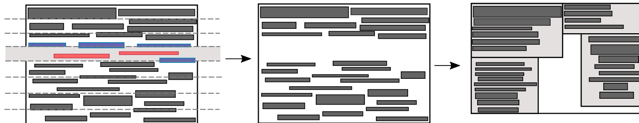
Figure 5.3: Obtaining containers from a box in two steps. First, we remove the strip (shaded in light grey) with least profit of items completely contained in it (shown in red). We also remove the items partially intersecting that strip (shown in blue. These will be constant in number). Then in the second step, we apply resource augmentation lemma to obtain constant number of containers.
